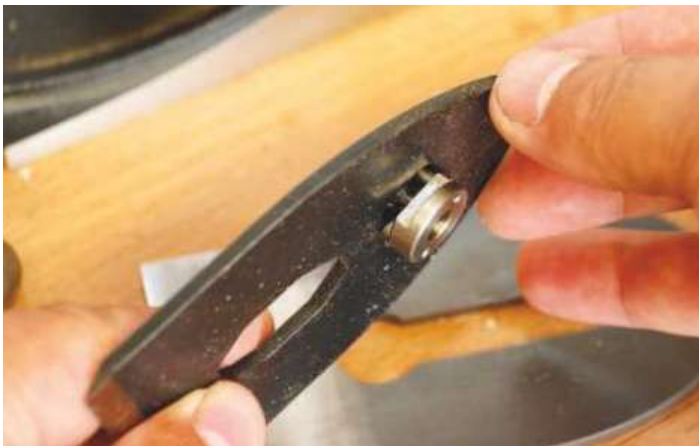
▲ The carrier is then held on the cap iron so both need to be nipped up when resetting
